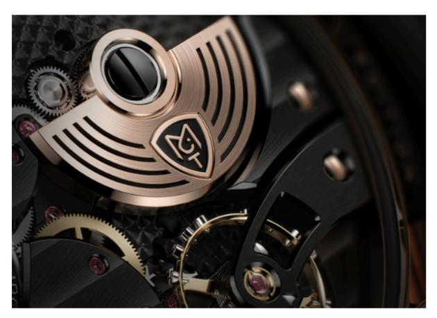
The new caliber benefits from the latest advances in teeth profiles on the gears. The high efficiency gears mean less energy wasted in friction losses, higher and more consistent power to the regulator for higher precision and a longer power reserve, while the lower mass of the micro-rotor requires less force than a traditional full-size rotor.
