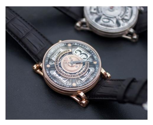
Its mechanism does features a small bridge, completing the circle, within which the gold selfwinding rotor oscillates. The mechanism consists of 507 parts, it's highly decorated and boasts hand-chamfered bridges, polished and adorned with circular Côtes de Genève motif; platinum is decorated with pearl graining. This high-end machine holds 40 hours of power reserve.
